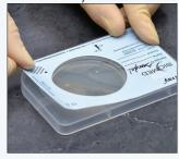
Reseal the InTray label to the plastic tray body. Press all around the perimeter of the InTray to ensure a complete seal.
